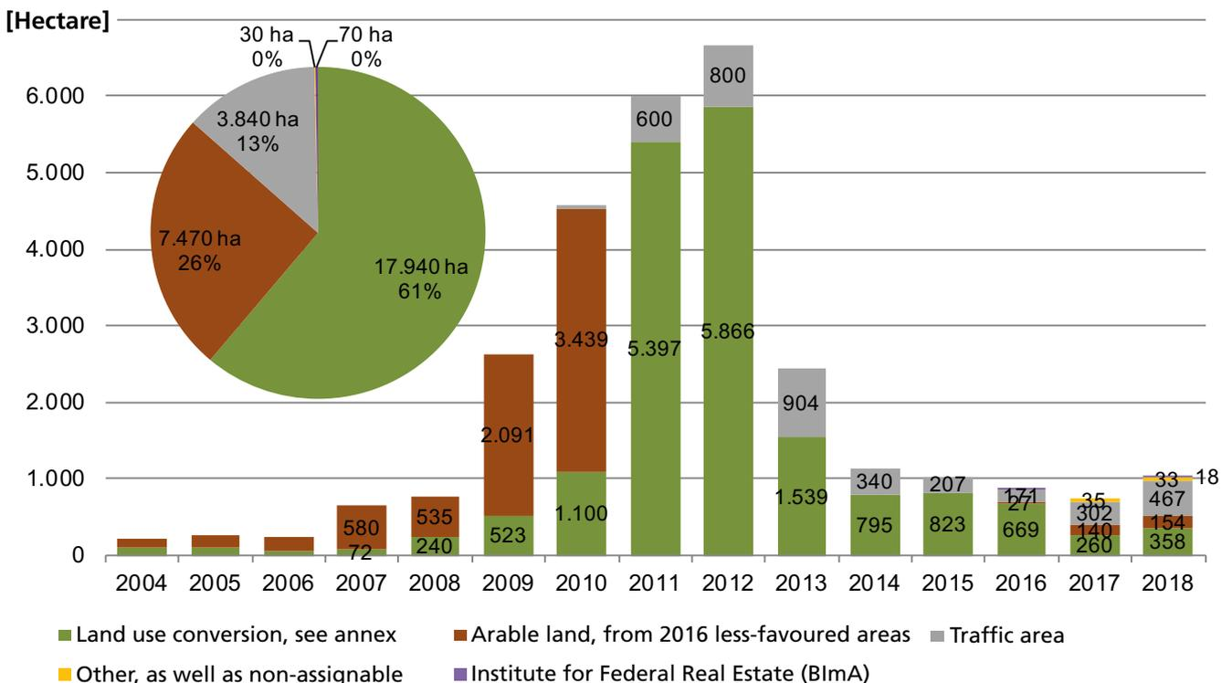
Figure 5: Land use for ground-mounted photovoltaic systems since 2004 in Germany, total portfolio and annual growth.<sup>[5]</sup> © BMWi
