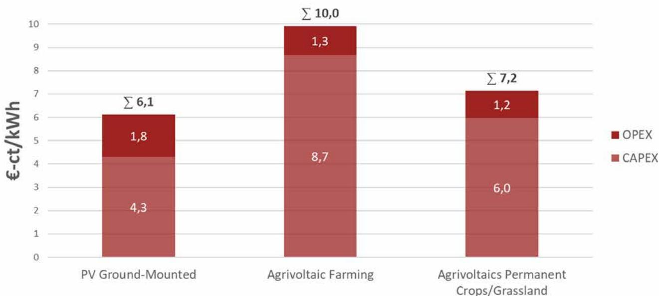
Figure 29: CAPEX / OPEX of ground-mounted photovoltaic systems and agrivoltaics in comparison. Data from [4, 22]
