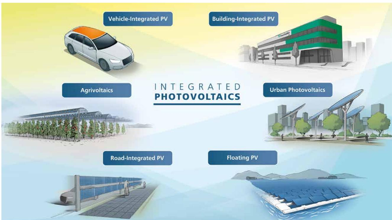
Figure 6: Applications for the integration of photovoltaics. © Fraunhofer ISE
