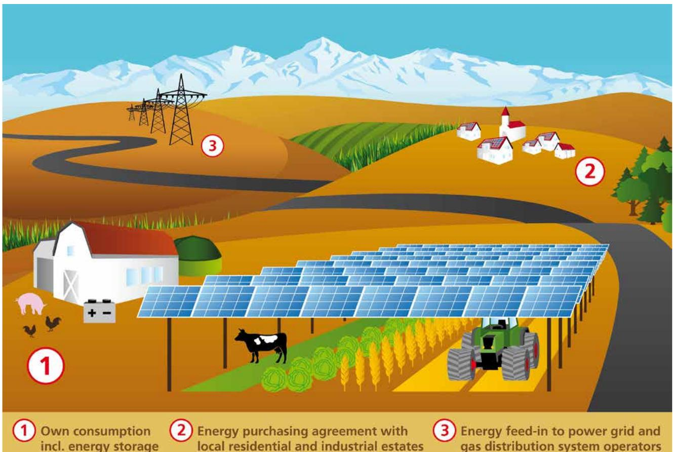
Figure 1: Illustration of an agrivoltaic system. © Fraunhofer ISE
