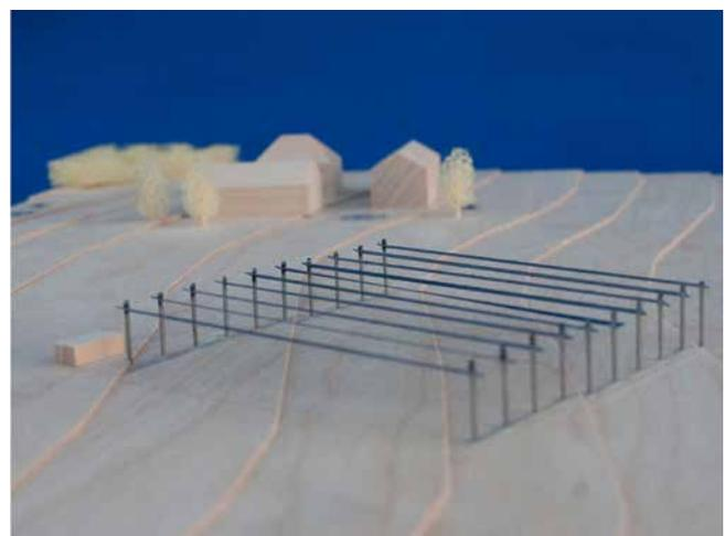
Figure 51: Model of the agrivoltaic system in Heggelbach for workshops. © Fraunhofer ISE
