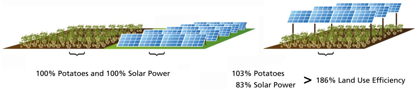
Figure 13: Through the combined use of land, the land use efficiency with agrivoltaics on the test site in Heggelbach is up to 186 percent. (Illustration of potatoes © HappyPictures/shutterstock.com)
