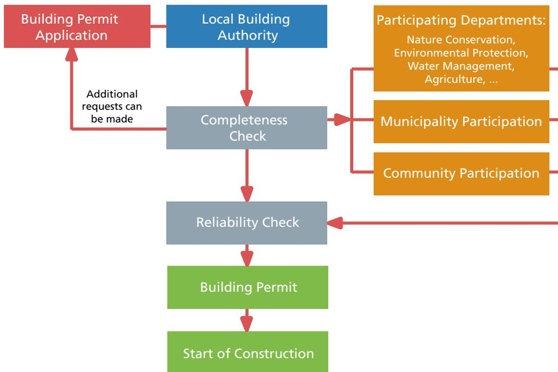
Figure 54: Example for the process of a building application.
