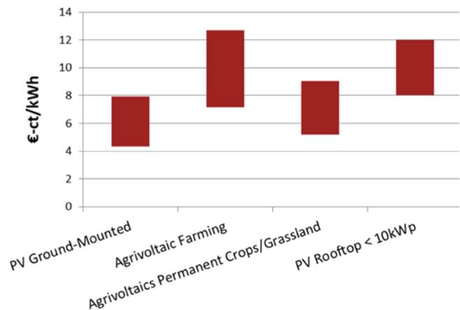
Figure 30: Estimated average levelized cost of electricity for ground-mounted photovoltaic systems and agrivoltaics, representation by Fraunhofer ISE, data from [3, 4, 23, 24]
