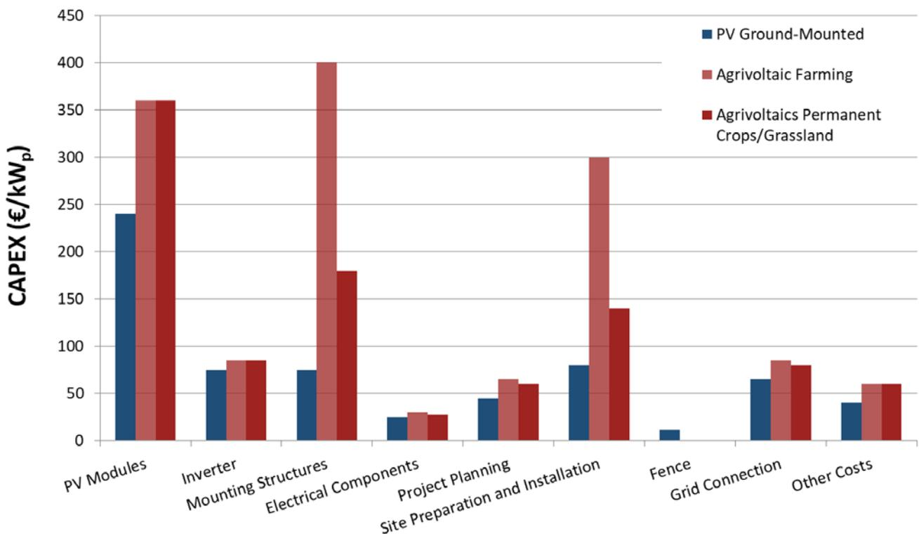
Figure 28: Investment costs for ground-mounted photovoltaic systems and agrivoltaics. Data from [4, 22]
