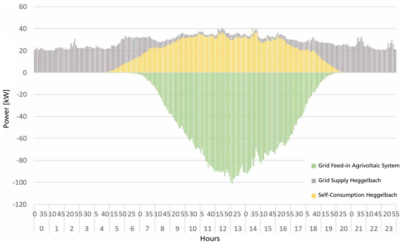
Figure 12: The Hofgemeinschaft Heggelbach was able to cover almost all its electricity needs with power generated by the agrivoltaic system in the summer of 2017. © BayWa r.e.
