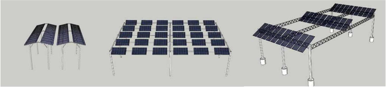
Figure 43: Illustration of different types of agrivoltaic systems with east-west, south- and south-east orientation. © Fraunhofer ISE
