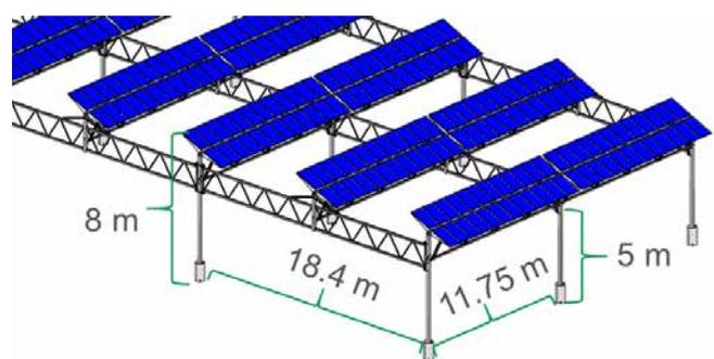
Figure 11: Sketch of the agrivoltaic reference plant in Heggelbach. © Hilber Solar
