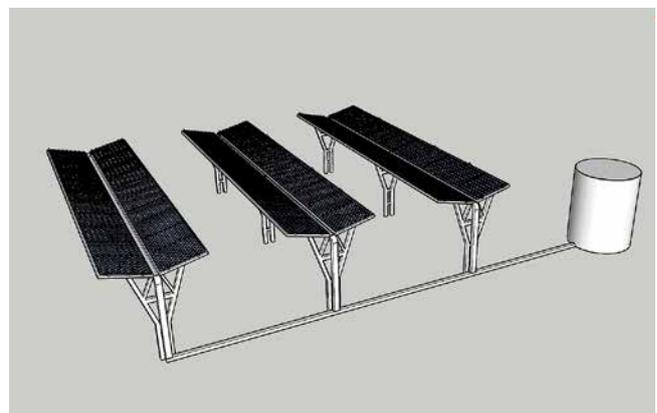
Figure 45: Concept of a rainwater harvest system with underground storage tank. © Fraunhofer ISE
