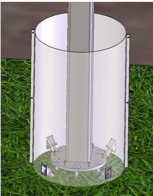
Figure 20: Fenders on the supports of the system in Heggelbach project against damage from farm machinery. © Hilber Solar
